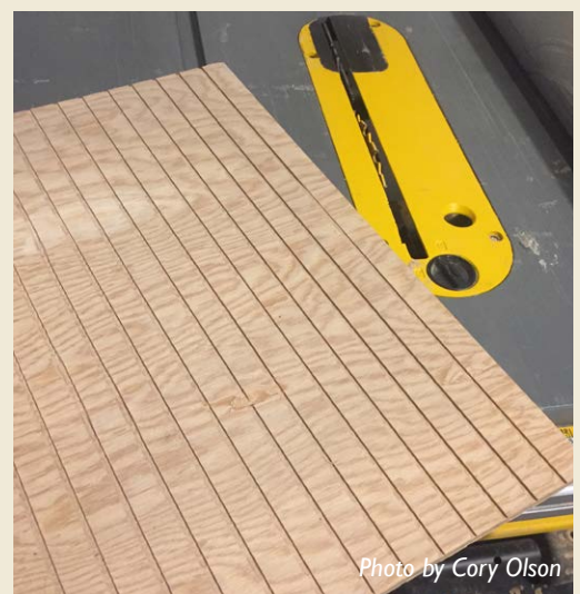
Horizontal grooves being cut using a table saw. These grooves allow bats to gain traction when climbing or resting.
