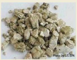
Vermiculite used to insulate homes has potential to contain asbestos fibres (a potentially harmful material). Be careful not to disturb this material when cleaning, and seek professional advice if it is present.
