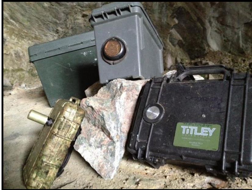
C. Lausen monitored Queen Victoria mine in West Kootenays this winter using the whole arsenal of Titley bat detectors as a way of comparing and testing the new Anabat Express, and at the same time verifying that all 3 bat species continued to use this newly gated mine. From left to right: AnabatExpress, Anabat SD2 (in housing with external battery housing in background), Roostlogger. Photo: C. Lausen
