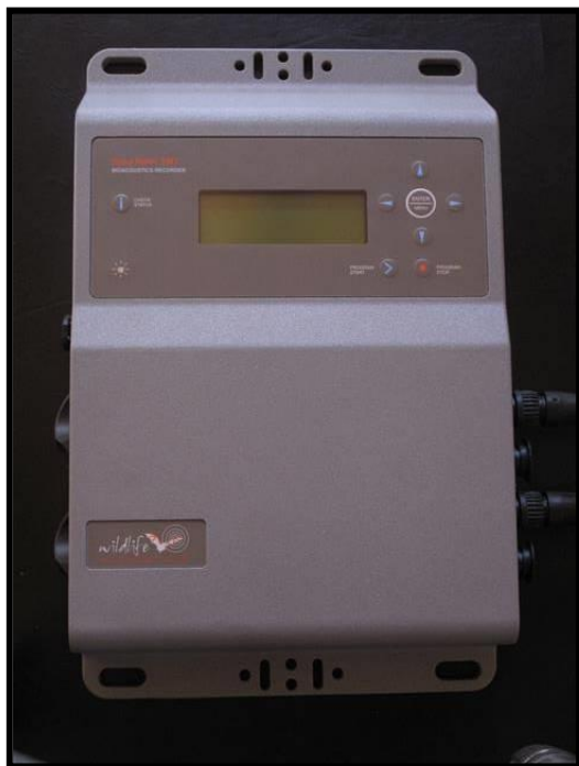
SM3BAT by Wildlife Acoustics. Not shown: 2 SM3-U1 microphones attached at ports bottom right. Photo: C. Lausen.
