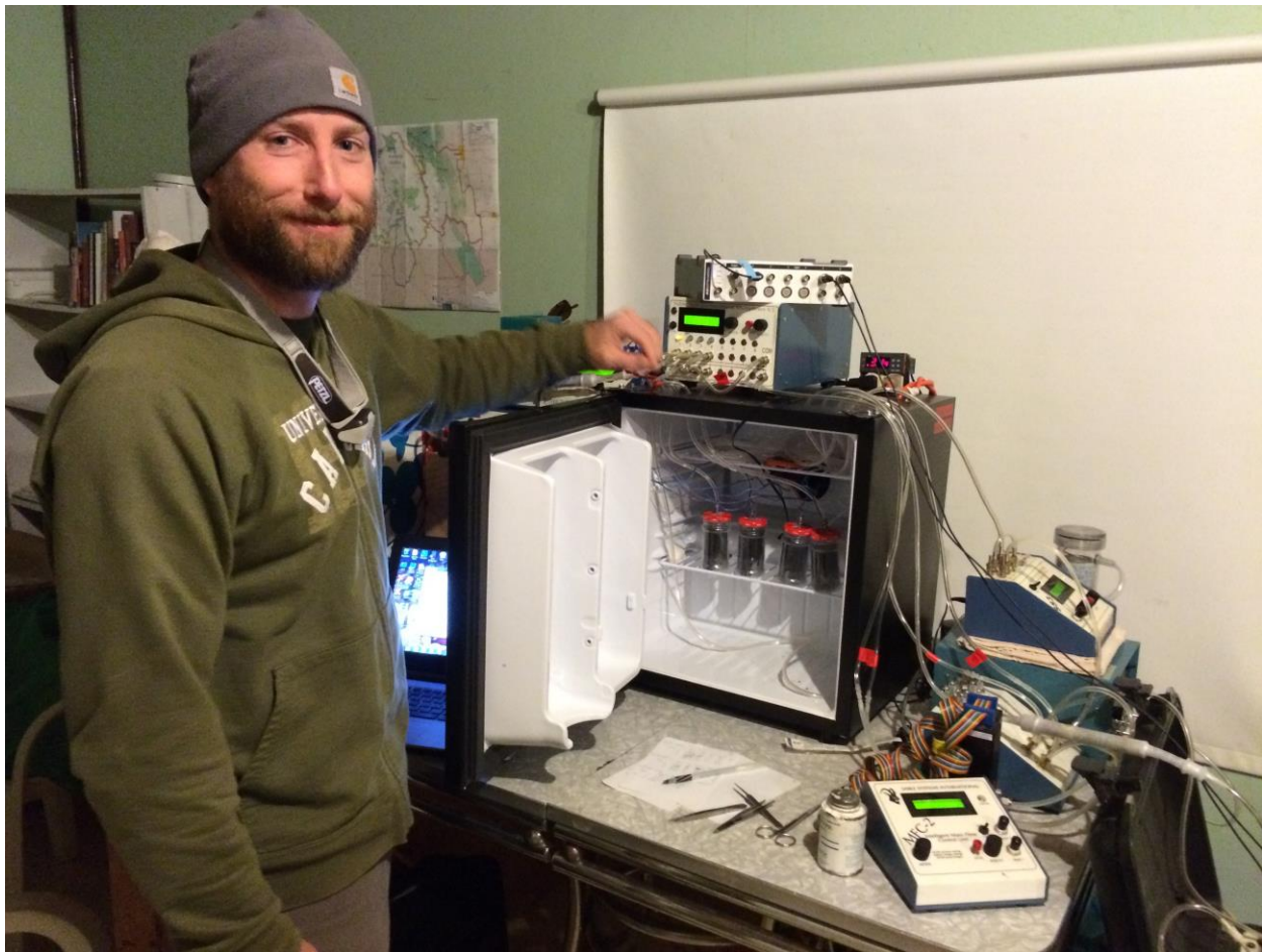
Brandon Klug, University of Regina, with respirometry chamber. Oxygen consumption of Myotis yumanensis (in 4 containers) was measured at experimental temperatures to determine metabolic rates and identify the lowest temperature at which bats are likely to hibernate. Photo by Michael Proctor.
