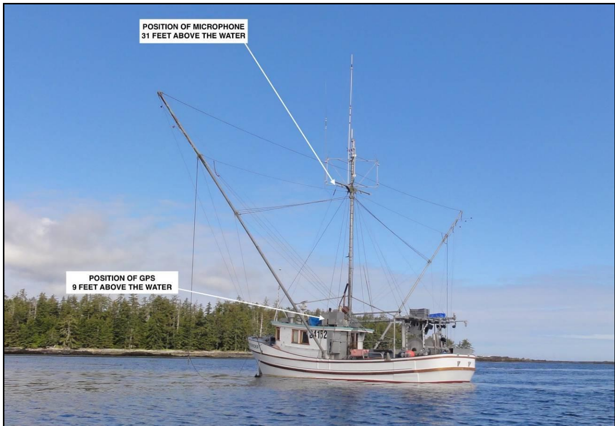
The Pacific Provider anchored off Cape Naden, Virago Sound, Haida Gwaii, British Columbia, showing the location of the microphone placement on the mast (@31 ft / 9.5 m), and GPS receiver (@9 ft / 2.75 m).
