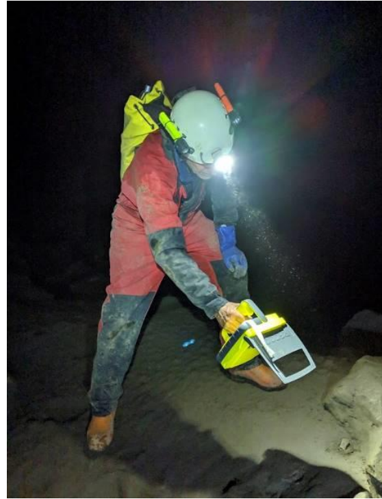
Greg Horne uses RECCO avalanche receiver in Cadomin Cave to look for modified ibuttons that have either fallen off of bats during the winter, or remain on bats that are still in the cave near the end of the hibernation period. Photo: Cory Olson.
